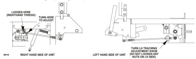
NOTE: The nut to the front of the unit on the RH rod has left-hand threads. FIGURE 17
